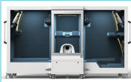
▲ Fig. 2 ATS1800C ultra compact CATR (center), with additional side chambers (ATS1800M) for multi-angle-of-arrival tests.
